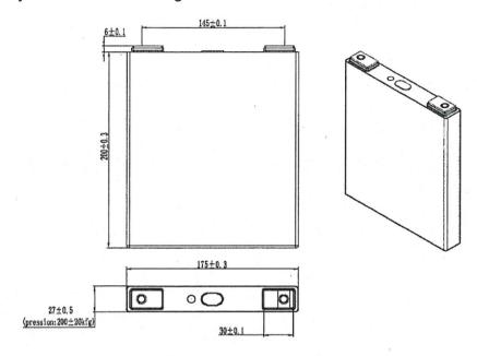
Figure A.1 Battery size diagram
